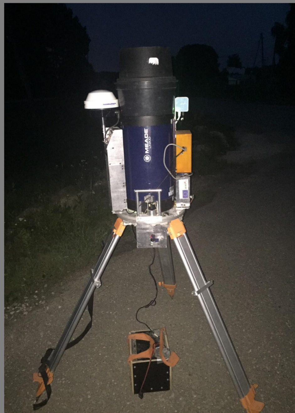
Figure 2. Digital Zenith Camera
