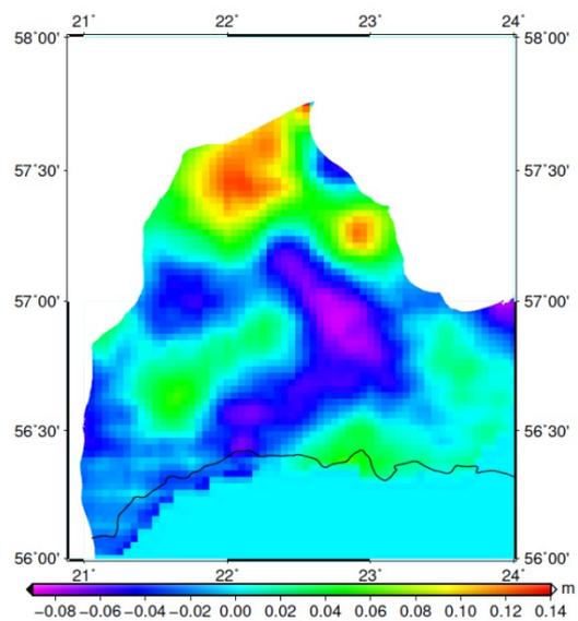
Fig. 6. The difference between LV98 and GNSS/levelling + VD + EGM2008 solution.
