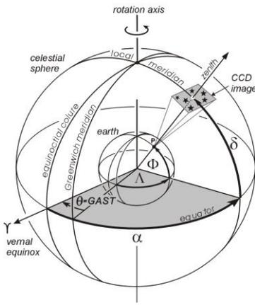
Fig. 1. Basic principle of the determination of the plumb line ( $\Phi$ ,  $\Lambda$ ) by imaging the stars in zenith direction [5].
