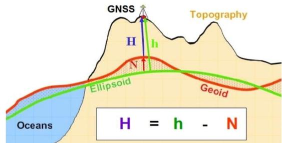
Fig. 4. The principle of GNSS-based height determination [16].
