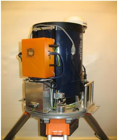
Fig. 3. Digital Zenith camera of Institute of Geodesy and Geoinformatics.
