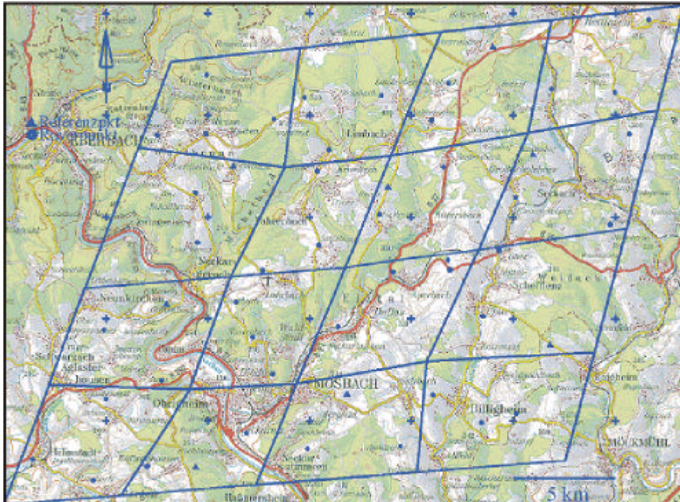
Figure 7. Meshing and data design of the identical points ( H,h ) of a DFHRS computation for the Mosbach region.
